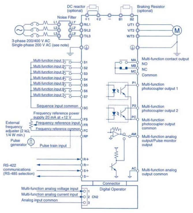
Note: Connect single-phase 230 VAC to terminals R/L1 and S/L2 of the 3G3MV-CB□.
